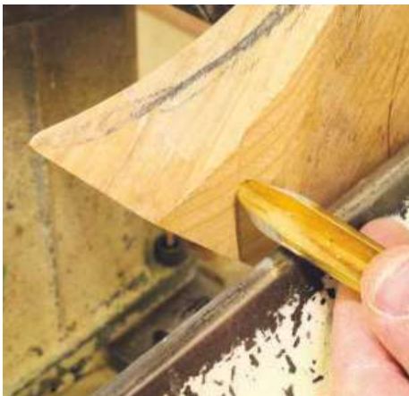
▲ Pic.22 The tool's flute position is critical here: if you have the flute too open and pointing upwards, you run the risk of catching the unsupported right hand cutting edge and breaking the piece. This photo shows the correct orientation
